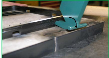
Replacing knife. Line up the cavity to the board and slowly tap in going around the perimeter of the knife. See below: (go in straight and perpendicular to board)
