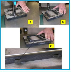
Use Green puller to place in bridged knife and pry slowly up by rocking back.(see arrow) Continue this around all the bridges by going around the perimeter. Remember to continue doing this in a straight and slow pattern. Damages to the board can occur if not done straight up.
